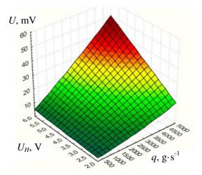
Fig. 4. Dependence of U output voltage from  $U_H$  supply voltage of bridge circuit and intensity of q milk ejection
