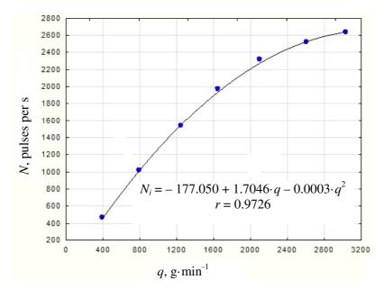
Fig. 5. Dependence of  $N_i$  number of impulses of measurement scheme of thermoanemometric measuring device on intensity of q milk ejection
