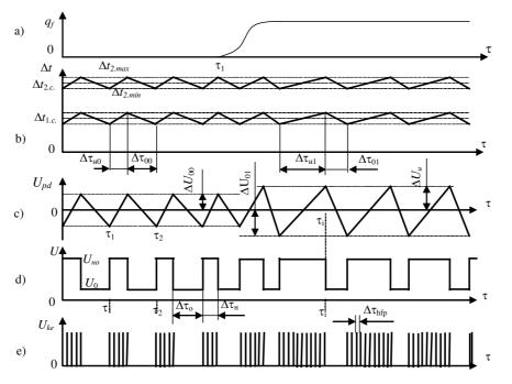
Fig. 2. Work diagrams of thermoanomometric counter of pulsating flow measuring device of two-phase medium:  $a - q_n$  milk ejection;  $b - \Delta t_1$  and  $\Delta t_2$  superheat temperature of thermistor elements; c – output voltage of 3 phase detector and input voltage of 4 null device; d – supply voltage of bridge circuit from the 10 square oscillation generator; e – characteristic of the output voltage of 5 electronic key
