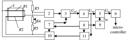
Fig. 1. Block scheme of thermoanemometric measuring device of pulsating flow of two-phase medium: 1 – body; R1, R2 – thermistor elements; R3, R4, R5 – resistors of bridge circuit; 2 – alternating current amplifier; 3 – phase detector; 4 – null device; 5 – electronic key; 6 – bus-bar former; 7 – reference generator; 8 – power conditioner; 9 – high frequency pulser; 10 – rectangular oscillation generator, 11 – control unit
