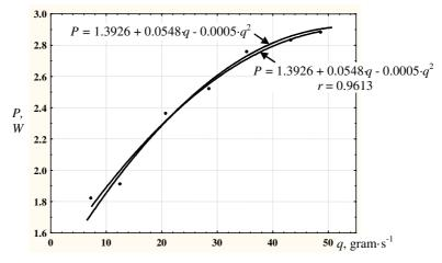
Fig. 3. Dependence of thermoanemometric sensor P measurement power on intensity of q milk ejection
